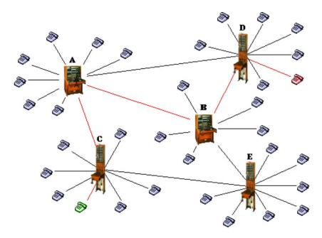
It shows switchboards for five exchanges labeled A, B, C, D, E. A number of phones are shown with direct connections to each switchboard. These would belong to customers located geographically near the associated switchboard's location. The diagram also shows connections between the switchboards. A is connected to D, B and C, but not to E. Switchboard E is connected to C and B but not to either A or D.
