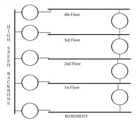
(b) The preceding design only has one backbone. So, if one of the routers connecting a floor to the backbone were to fail, the network would have to route traffic from that floor to other floors through either the floor above or below where the failure occurred. To make the network even more tolerant of failure, we might consider adding a backup backbone. That is, we will add a second backbone network and connect it to the floor networks with bridges as shown below.
