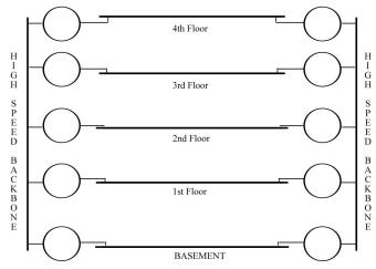
The hope would be that if one of the bridges connected to the primary backbone failed, the traffic would be shifted to the added backbone. It would also be nice, of course, if during normal operation the two backbones could share the load. Explain why neither of these goals is attainable using the transparent bridge spanning tree algorithm.
