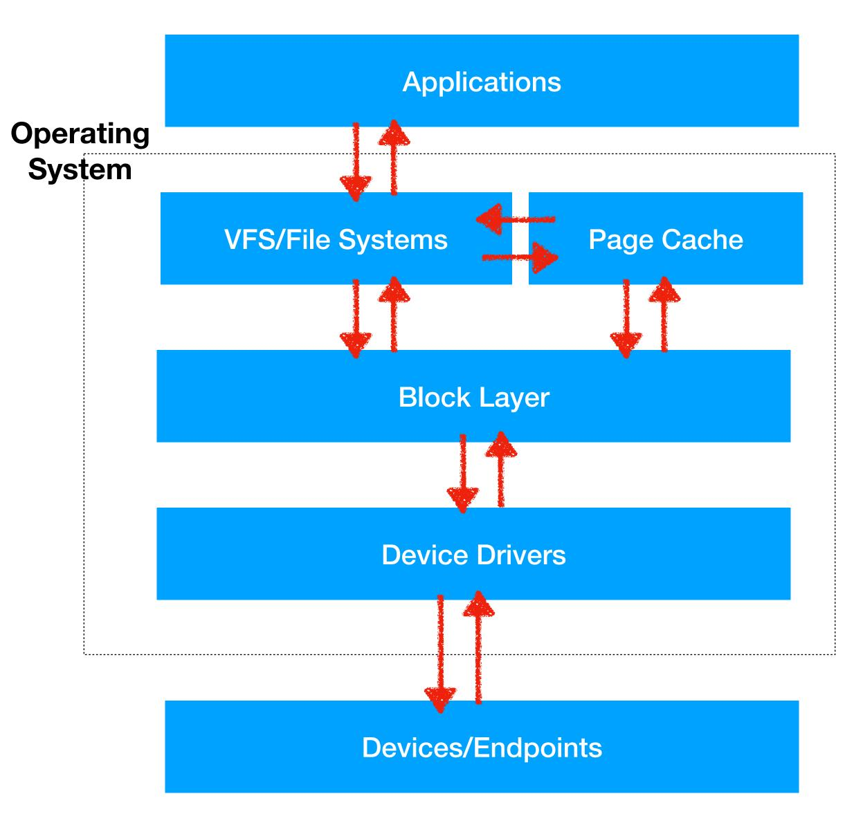
The Operating System consists of a series of interacting layers.
