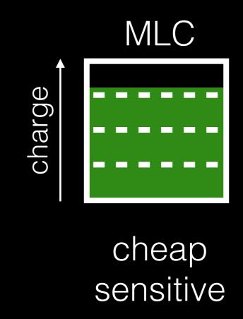
TLC (3 bits/cell) and QLC (4 bits/cell) also exist, and are even cheaper and more sensitve than MLC.
