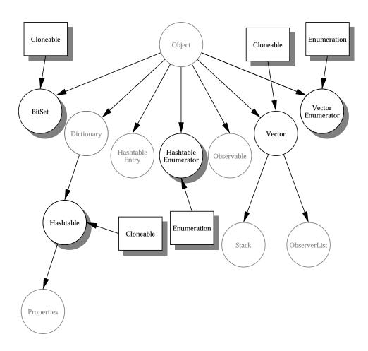
In this illustration, interfaces are represented by rectangles. You see that the Cloneable interface is implemented by multiple classes. In addition, the HashtableEnumerator and the VectorEnumerator classes both implement
