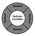
An object's *behavior* is defined by its *methods*. Methods manipulate the instance variables to create new state; an object's methods can also create new objects.
