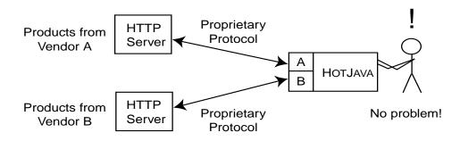
Protocol handlers get installed in a sequence similar to how content handlers get installed: The HotJava Browser is given a reference to an object (a URL). If the handler for that protocol is already loaded, it will be used. If not, the HotJava Browser will search first the local system and then the system that is the target of the URL.
