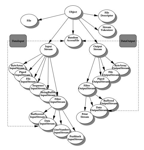
Note that the grayed out boxes with DataInput and DataOutput represent interfaces, not classes. Any new I/O class that subclasses one of the other classes can implement the appropriate interface if it needs to.
