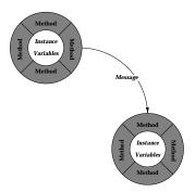
If an object wants another object to do some work on its behalf, then in the parlance of object-oriented programming, the first object sends a *message* to the second object. In response, the second object selects the appropriate *method* to invoke. Java method invocations look similar to functions in C and C++.
