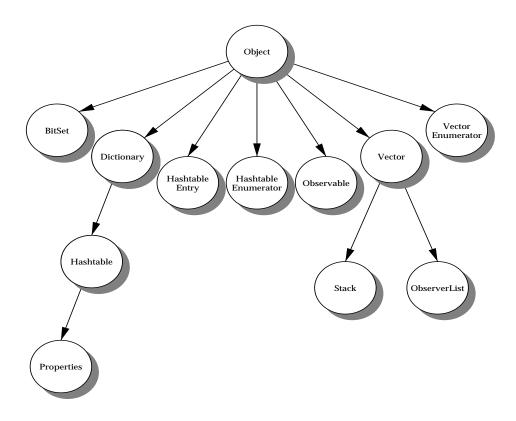
However, the above diagram points out the minor weakness with the single-inheritance model. Notice that there are two different kinds of *enumerator* classes in the picture, both of which inherit from Object. An enumerator class
