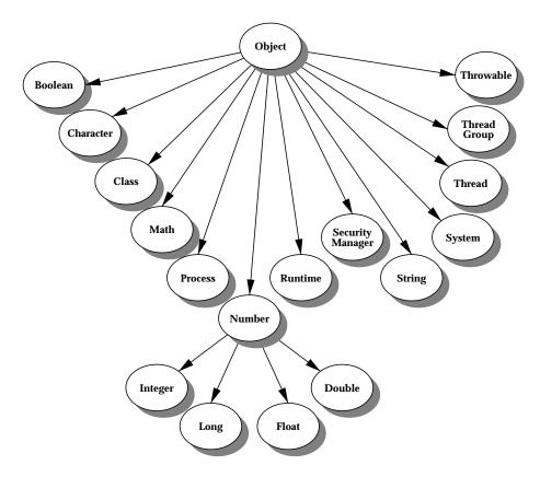
Note the Boolean, Character, and Number classes—these classes are "wrapper" classes for the primitive types. You use these classes in applications where the primitive types must be stored as objects. Note also the Throwable class—this is the root class for all exceptions and errors.
