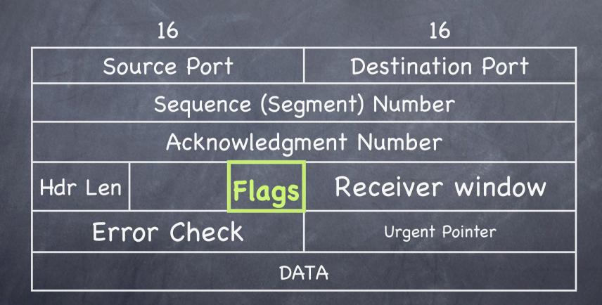
The Flags field of the TCP packet is used to distinguish special packets like the starting SYN packets.
