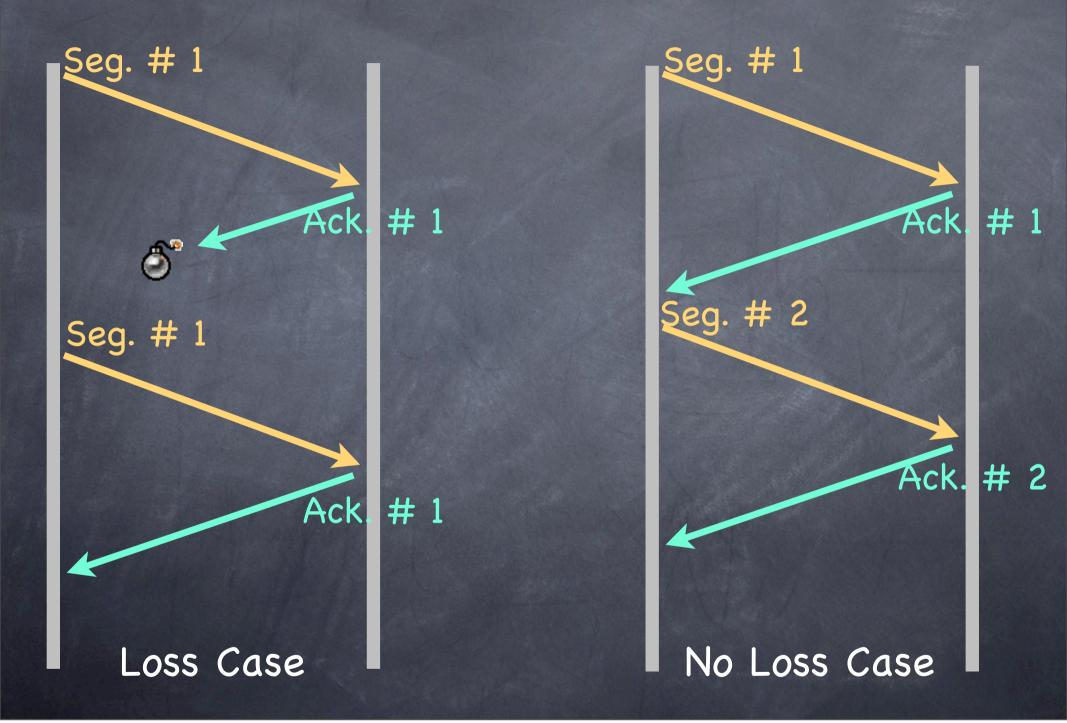
and the basic idea of using acknowledgment and retransmissions to ensure reliable delivery.
