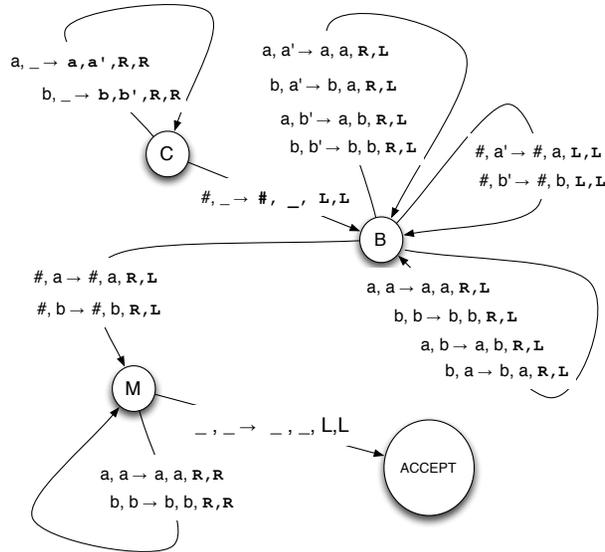
– The machine would start with the input on its first tape and nothing on the other.
