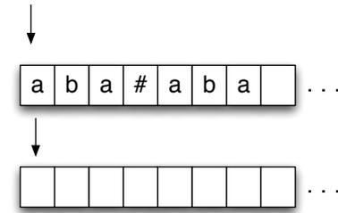
– It would first scan the input from left to right copying symbols from the input tape to the machine's second tape until reaching a  $\#$ . This is the role of state C = COPY.
