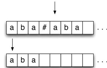
– Finally, it scans right on both tapes at the same time making sure that the contents of the second tape matches the contents of the second half of the input/first tape. This is the role of
