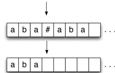
– Next, it moves the head on the second tape back to the left end of the tape (We would like to keep the head on the first tape right where it is, but since my version of n-tape TMs require each head to move left or right at each step, we have to make it wiggle back and forth). This is the role of state B = BACKUP.
