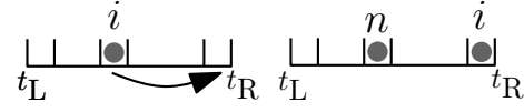
Figure 1: Case 1 from the proof of Lemma 6. Job i can be scheduled in t_R , and job n can be scheduled in t_i where i was previously.
