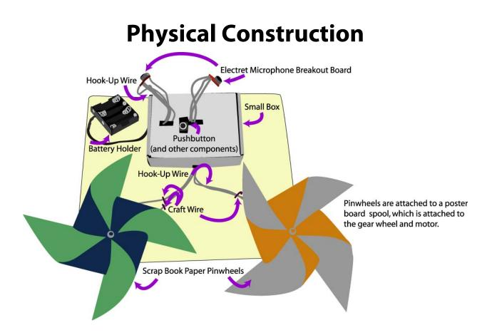
The above illustration shows the exterior of the Talk-O-Matic, and how the components fit together. The pinwheel mechanisms are made of several parts as well, as shown below.
