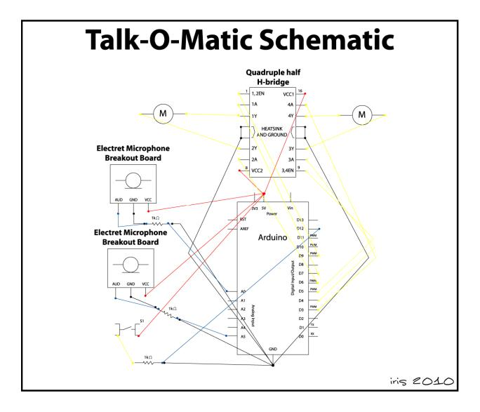
Below is a Fritzing Diagram of the Talk-O-Matic electronics components. The microphone breakout boards and the gear motors are attached to the breadboard, but are on the exterior of the Talk-O-Matic's small cardboard box. The rest of the electronics components attached to the breadboard and Arduino are stored inside the small box.
