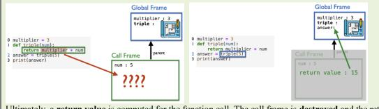
Ultimately, a **return value** is computed for the function call. The call frame is **destroyed** and the return value of the function call is assigned to the variable on the lefthand side of the assignment operator in the global frame.
